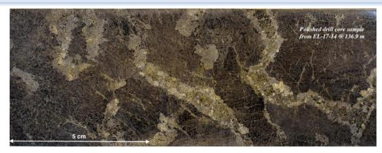
Loop textured massive pyrrhotite-pentlanditechalcopyrite, granular pentlandite and chalcopyrite grains forming on larger pyrrhotite grains
