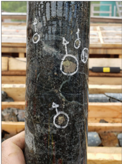
Hole EL-19-48 ~97m Blebbly pyrrhotite -pentlandite-chalcopyrite (Way-up lineation) Orbicular textured taxite
